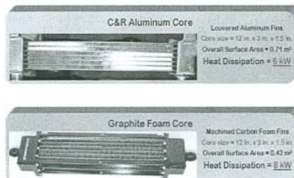
Aluminum Core and Graphite Foam Core Automotive Radiators
